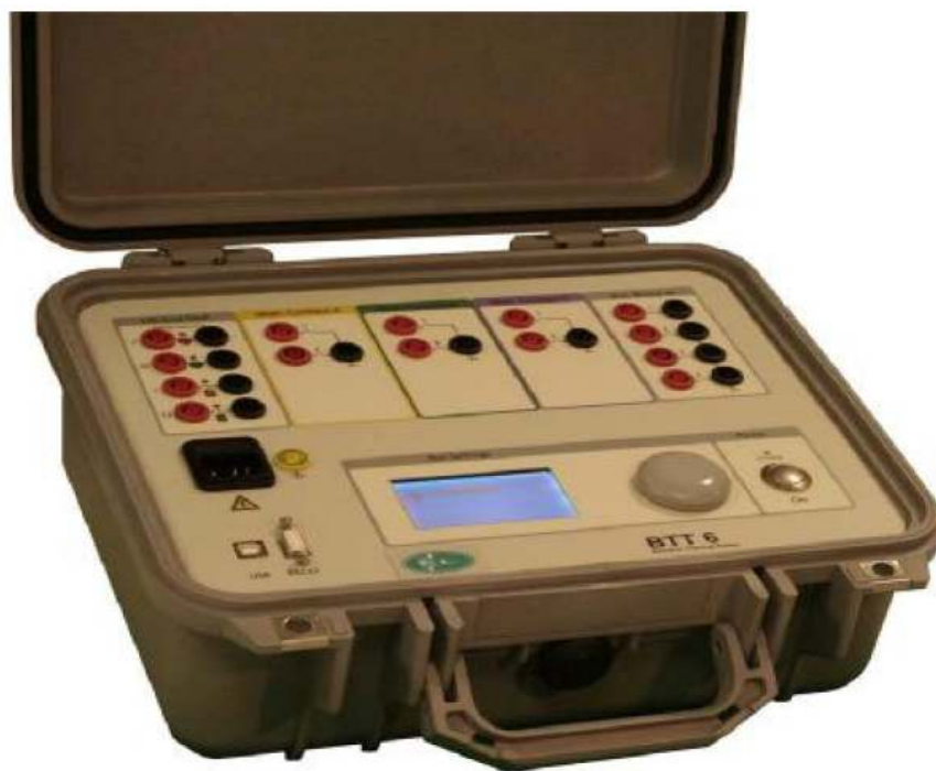
Rys. 3.1. Breaker Timing Tester ( tester BTT 6)
