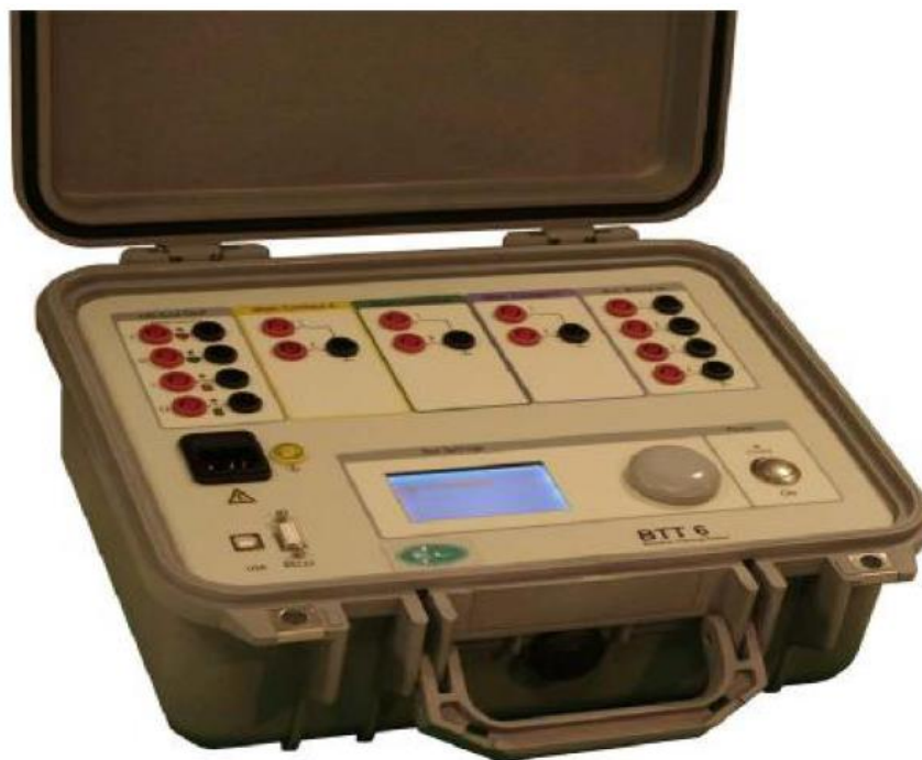
Rys. 3.1. Breaker Timing Tester ( tester BTT 6)
